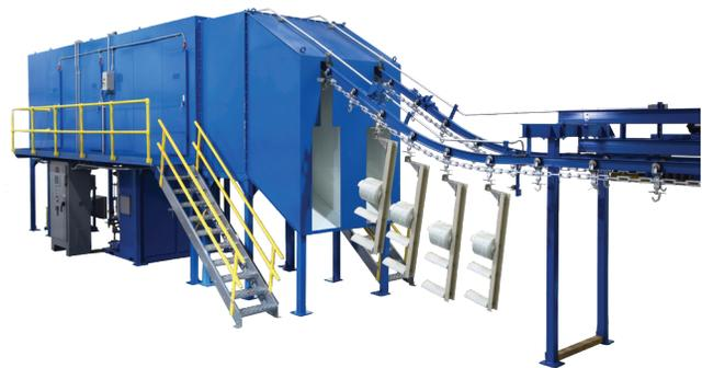
**100 KW RF Fiberglass Dryer**
